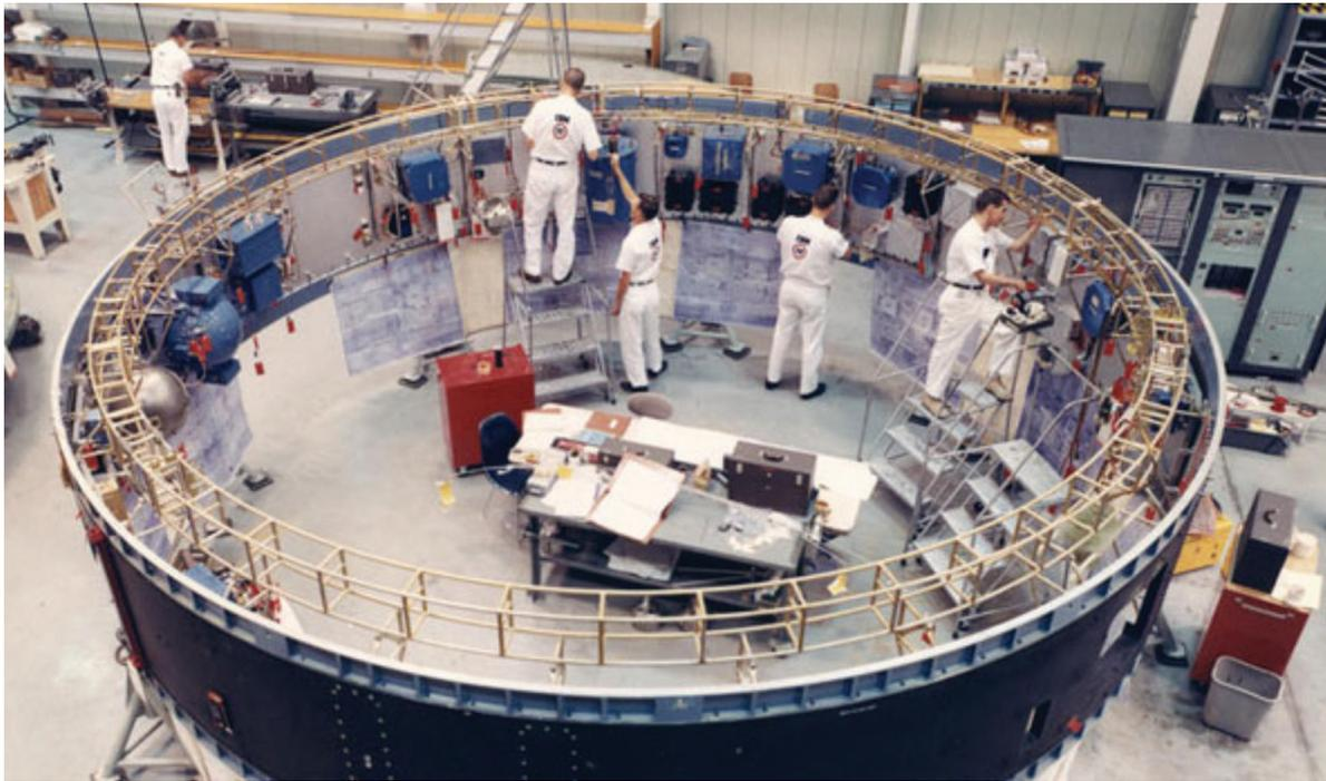
**Figure 2.** Manufacturing the Saturn V Instrument Unit. Credit: <https://www.ibm.com/ibm/history/ibm100/us/en/icons/apollo/breakthroughs/> Retrieved 7/22/2021
